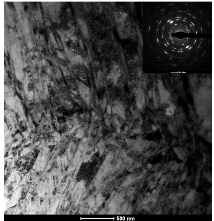
Fig. 3. A bright field TEM images with corresponding SAED patterns, transverse cross-section
