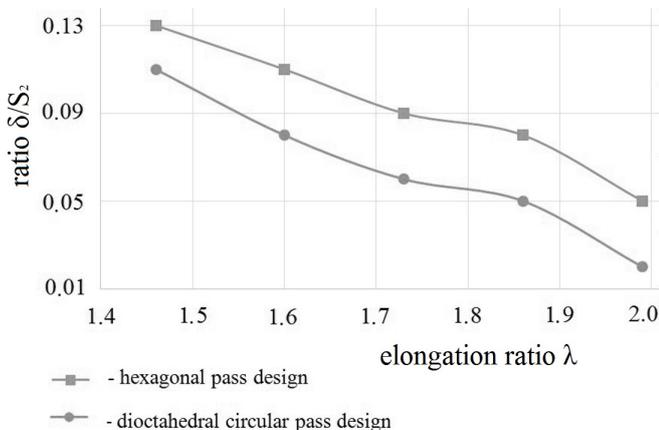
Fig. 7. Dependence of  $\delta/S_2$  ratio from elongation ratio  $\lambda$
