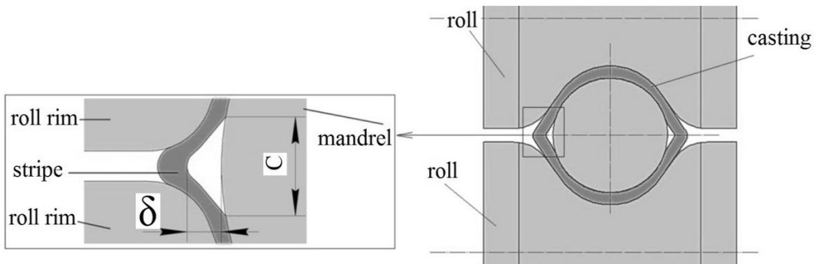
Fig. 5. Scheme for the determination of  $\delta$  and  $C$  ratios
