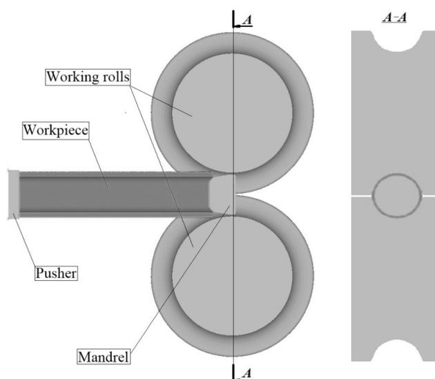
Fig. 2. Scheme of the plug rolling mill
