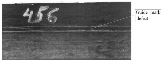
Fig. 1. Guide mark defect on the internal surface of the pipe
