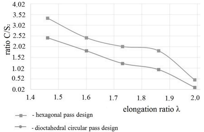
Fig. 8. Dependence of  $C/S_2$  ratio from elongation ratio  $\lambda$
