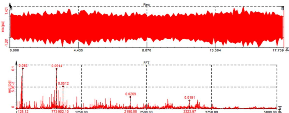
Fig. 2. AE signal of Good bearing
