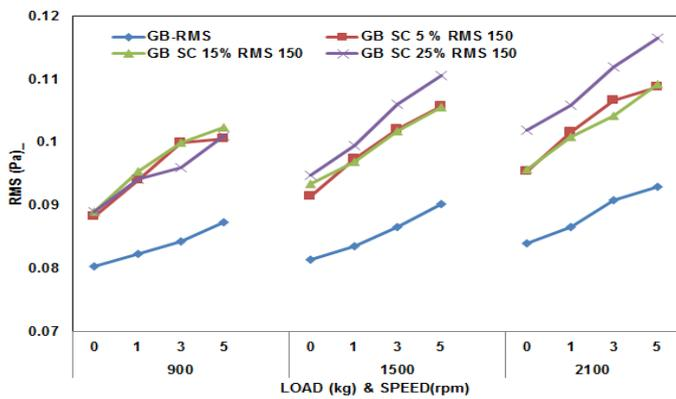
Fig. 3c. RMS graph for 150  $\mu\text{m}$  particle size
