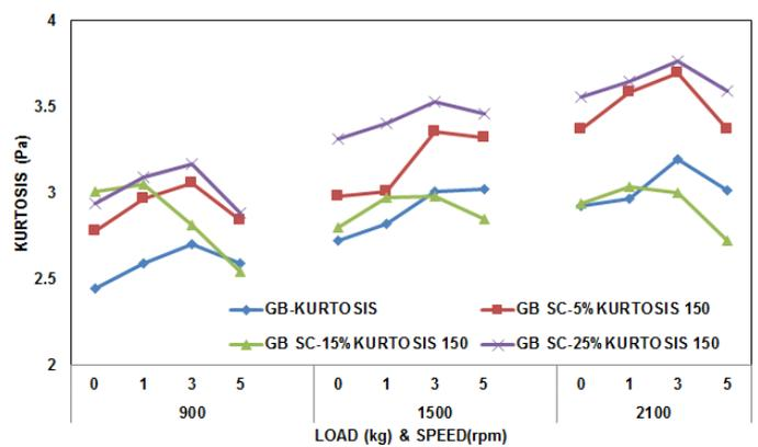
Fig. 4c. KURTOSIS graph for 150  $\mu\text{m}$  particle size
