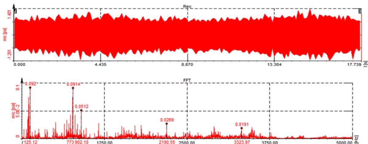
Fig. 2. AE signal of Good bearing
