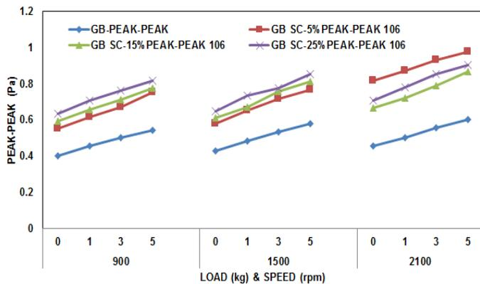
Fig. 5b. PEAK TO PEAK graph for 106  $\mu\text{m}$  particle size
