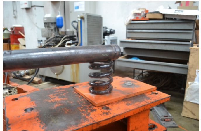
Fig. 2. Reinforcement of the free end of branch pipe by spring
