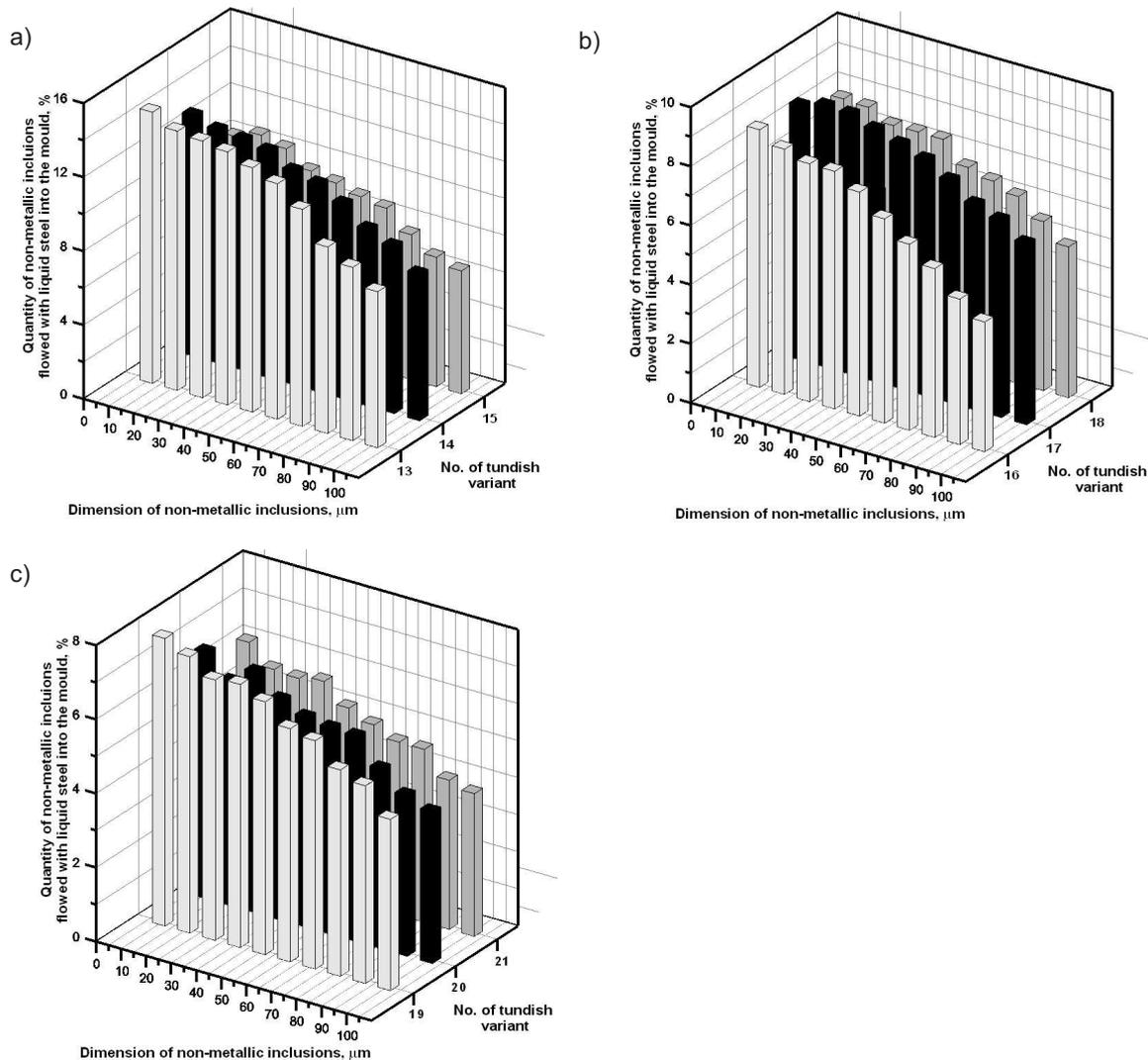
Fig. 7. Fraction of non-metallic inclusions flowed with liquid steel into the mould: a) variants nos. 13-15 of tundish modification, b) variants nos. 16-18 of tundish modification, c) variants nos. 19-21 of tundish modification
