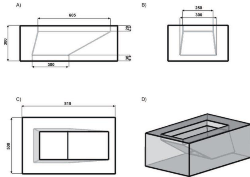
Fig. 4. Subflux turbulence controller no. 2
