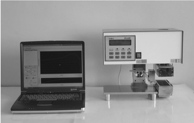
Fig. 1. Prototype apparatus DMA for measuring the distortion in high temperature [8]
