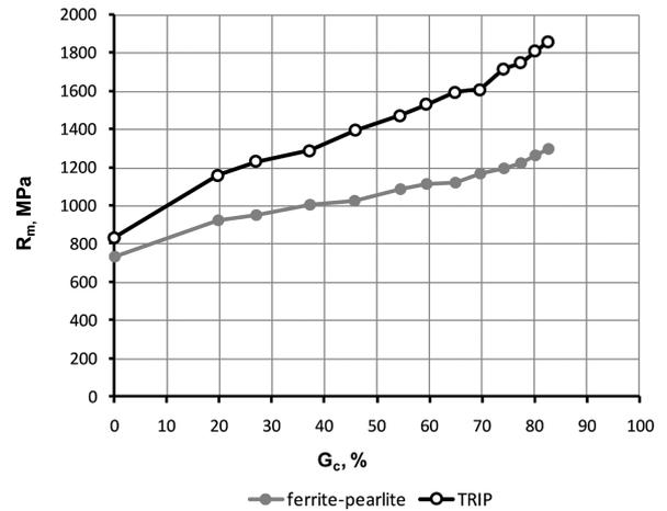
Fig. 13. Variation of the  $R_m$  tensile strength of wires made of TRIP steel and wires made of ferritic-pearlitic structure steel not heat treated (without the TRIP effect), drawn with small partial reductions and at a drawing speed of  $v=1.11$  m/s, as a function of the total reduction in area [10]
