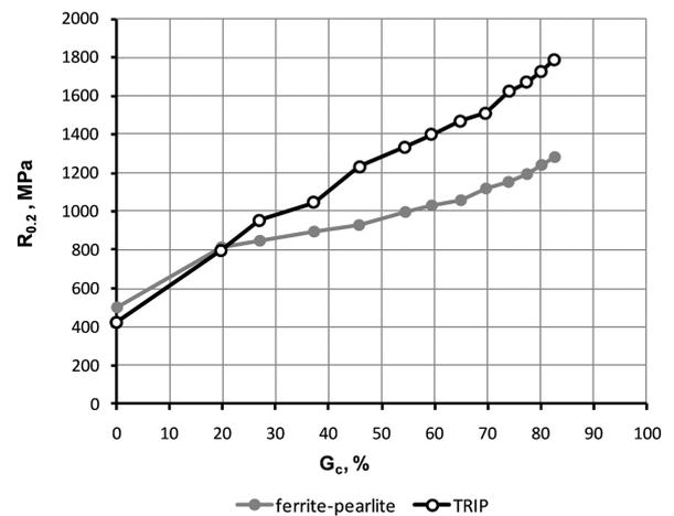
Fig. 14. Variation of the  $R_{0.2}$  yield strength of wires made of TRIP steel and wires made of ferritic-pearlitic structure steel not heat treated (without the TRIP effect), drawn with small partial reductions and at a drawing speed of  $v=1.11\text{ m/s}$ , as a function of the total reduction in area [10]
