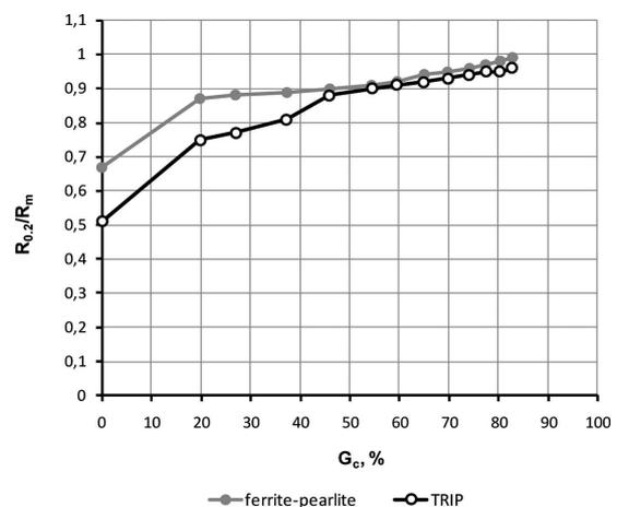
Fig. 15. Variation of the  $R_{0.2}/R_m$  ratio of wires made of TRIP steel and wires made of ferritic-pearlitic structure steel not heat treated (without the TRIP effect), drawn with small partial reductions and at a drawing speed of  $v=1.11\text{ m/s}$ , as a function of the total reduction in area [10]
