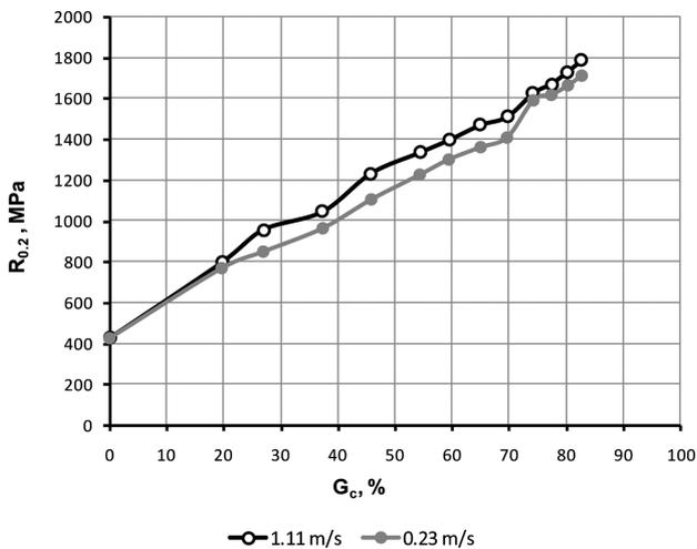
Fig. 9. Variation in the  $R_{0.2}$  yield strength of TRIP steel wires drawn with large partial reductions and at a drawing speed of  $v_1 = 1.11$  m/s and  $v_2 = 0.23$  m/s, respectively, as a function of the total reduction in area [10]
