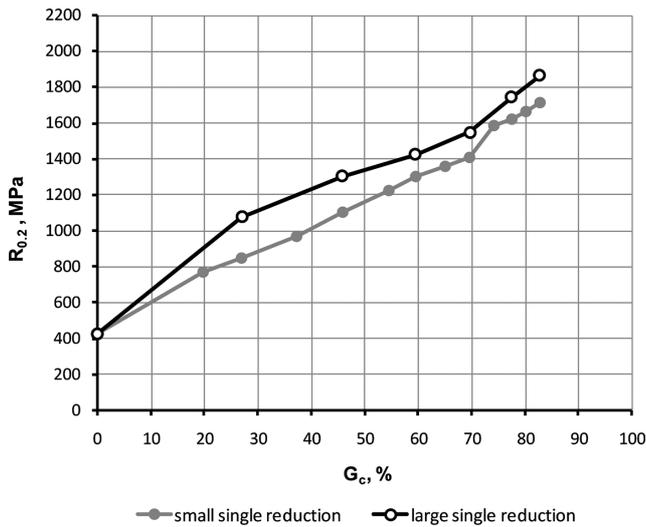
Fig. 4. Variation in the yield strength  $R_{0.2}$  of TRIP steel wires drawn with small and large partial reductions, respectively, at a drawing speed of 0.23 m/s, as a function of the total reduction in area [10]
