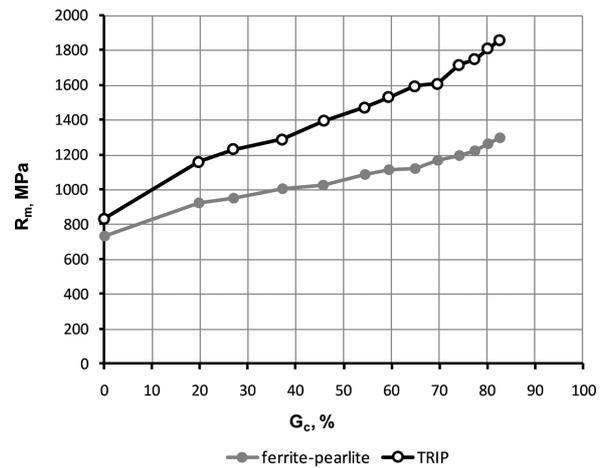
Fig. 13. Variation of the  $R_m$  tensile strength of wires made of TRIP steel and wires made of ferritic-pearlitic structure steel not heat treated (without the TRIP effect), drawn with small partial reductions and at a drawing speed of  $v=1.11\text{ m/s}$ , as a function of the total reduction in area [10]
