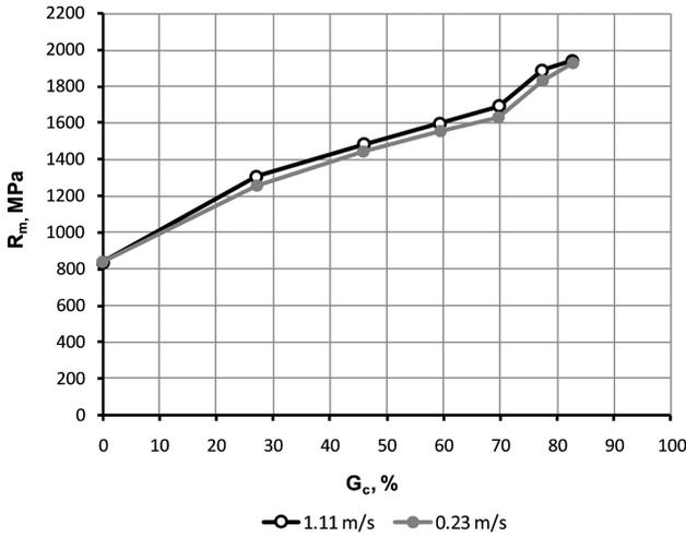
Fig. 8. Variation in the  $R_m$  tensile strength of TRIP steel wires drawn with large partial reductions and at a drawing speed of  $v_1 = 1.11$  m/s and  $v_2 = 0.23$  m/s, respectively, as a function of the total reduction in area [10]
