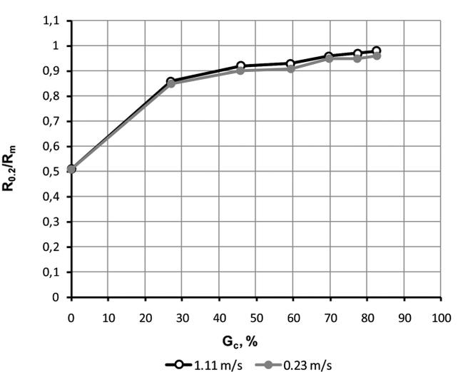
Fig. 12. Variation in the  $R_{0.2}/R_m$  ratio of TRIP steel wires drawn with large partial reductions and at a drawing speed of  $v_1 = 1.11$  m/s and  $v_2 = 0.23$  m/s, respectively, as a function of the total reduction in area [10]
