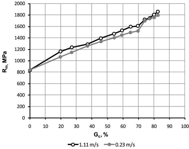
Fig. 7. Variation in the  $R_m$  tensile strength of TRIP steel wires drawn with small partial reductions and at a drawing speed of  $v_1 = 1.11$  m/s and  $v_2 = 0.23$  m/s, respectively, as a function of the total reduction in area [10]
