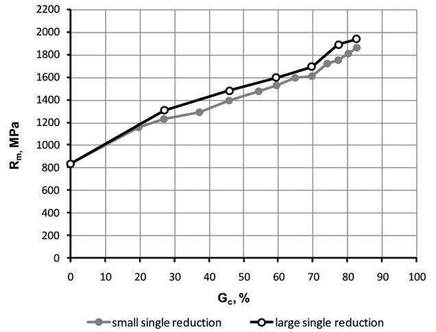
Fig. 1. Variation in the ultimate tensile strength  $R_m$  of TRIP steel wires drawn with small and large partial reductions, respectively, at a drawing speed of 1.11 m/s, as a function of the total reduction in area [10]
