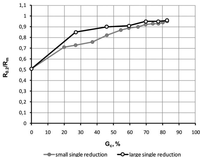
Fig. 6. Variation in the  $R_{0.2}/R_m$  ratio for TRIP steel wires drawn with small and large partial reductions, respectively, at a drawing speed of 0.23 m/s, as a function of the total reduction in area [10]
