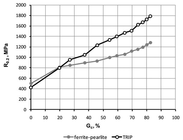
Fig. 14. Variation of the  $R_{0.2}$  yield strength of wires made of TRIP steel and wires made of ferritic-pearlitic structure steel not heat treated (without the TRIP effect), drawn with small partial reductions and at a drawing speed of  $v=1.11$  m/s, as a function of the total reduction in area [10]
