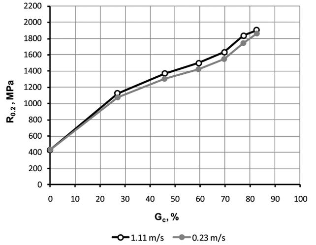
Fig. 10. Variation in the  $R_{0.2}$  yield strength of TRIP steel wires drawn with large partial reductions and at a drawing speed of  $v_1 = 1.11$  m/s and  $v_2 = 0.23$  m/s, respectively, as a function of the total reduction in area [10]
