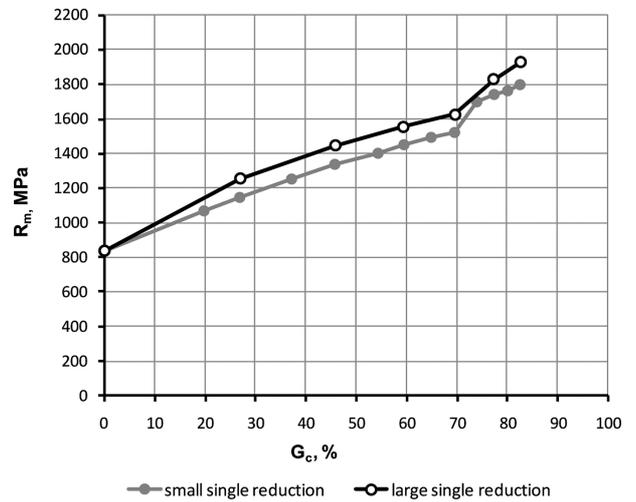
Fig. 2. Variation in the ultimate tensile strength  $R_m$  of TRIP steel wires drawn with small and large partial reductions, respectively, at a drawing speed of 0.23 m/s, as a function of the total reduction in area [10]
