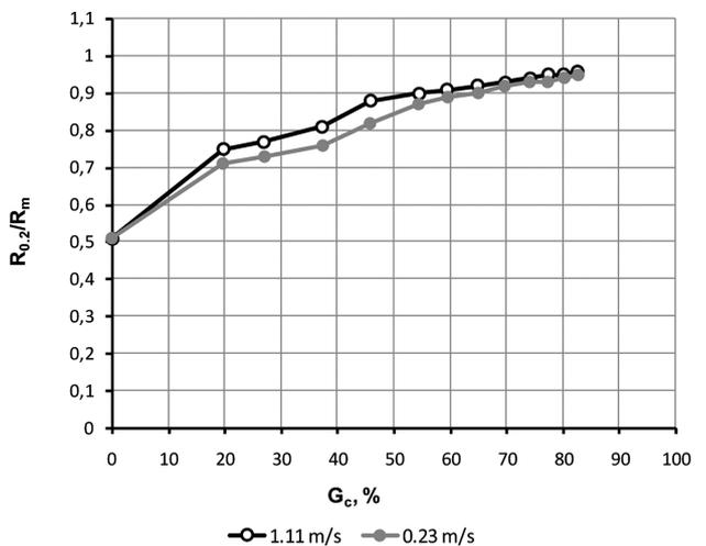
Fig. 11. Variation in the  $R_{0.2}/R_m$  ratio of TRIP steel wires drawn with small partial reductions and at a drawing speed of  $v_1 = 1.11$  m/s and  $v_2 = 0.23$  m/s, respectively, as a function of the total reduction in area [10]
