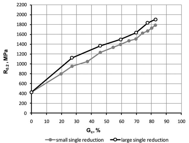
Fig. 3. Variation in the yield strength  $R_{0.2}$  of TRIP steel wires drawn with small and large partial reductions, respectively, at a drawing speed of 1.11 m/s, as a function of the total reduction in area [10]
