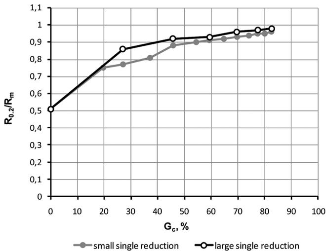
Fig. 5. Variation in the  $R_{0.2}/R_m$  ratio for TRIP steel wires drawn with small and large partial reductions, respectively, at a drawing speed of 1.11 m/s, as a function of the total reduction in area [10]
