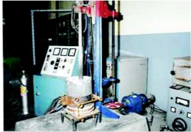
Fig. 2. Laboratory EAF – Test stand
