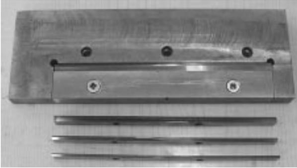
Fig. 3. Tool segment used in experimental research of CWR in cold forming conditions
