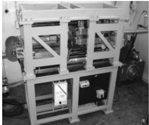
Fig. 2. Laboratory stand LUW-2 for CWR with two flat wedges
