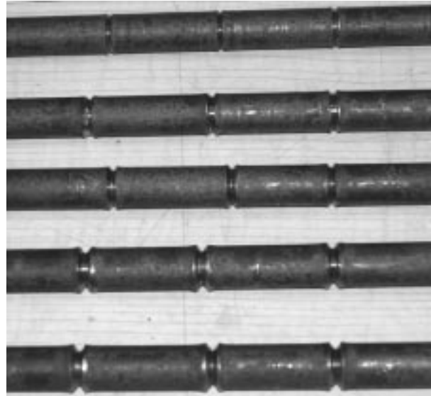
Fig. 4. Samples with V – grooves obtained in the CWR processes at: \alpha = 50^\circ and \Delta r = 1.0; 1.6; 2.0; 2.6 and 2.9 mm (from the top)
