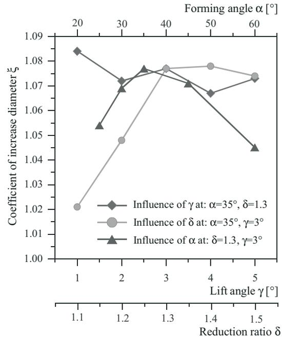
Fig. 11. Calculated by means of FEM the influence of wedge angles ( $\alpha, \gamma$ ) and reduction ratio  $\delta$  on the increase of diameter of parts formed in free CWR at  $d_0 = 30$  mm and  $m = 0,9$
