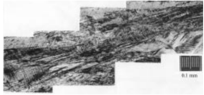
Fig. 15. Localized strain band for bronze CuSi3.5 at ambient temperature after tension ( \dot{\epsilon}_{pr} = 0.01 \text{ s}^{-1} ) with simultaneous cyclic torsion ( \dot{\epsilon} = 0.1 \text{ s}^{-1} ) at amplitude of 0.11 to equivalent strain of 0.8 at ambient temperature
