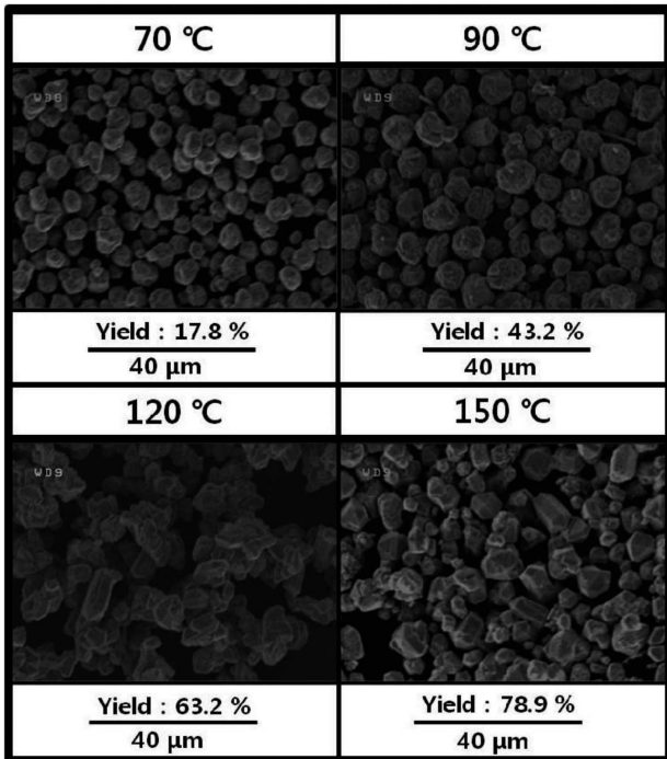
Fig. 4. SEM images and yields of Cu powders synthesized in an ethylene glycol for 3 h at different temperatures
