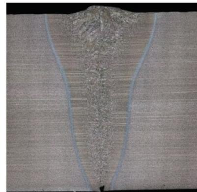
Fig. 6. Macrostructure of the Weldox 1300 steel EBW joint
