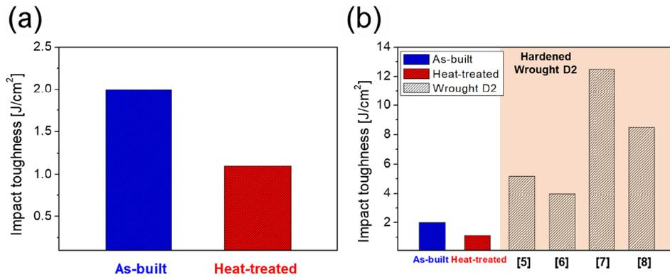
Fig. 2. (a) Impact toughness results of the DED as-built and DED heat-treated AISI D2 steels, and (b) comparison results between DED AISI D2 materials and other conventional wrought AISI D2 materials
