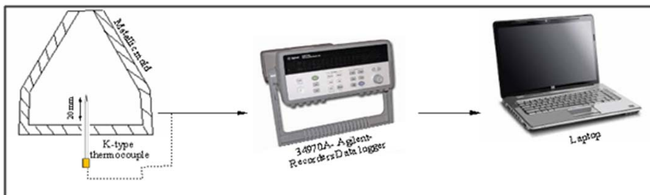
Fig. 2. Thermal analysis configuration with metallic mold and a thermocouple
