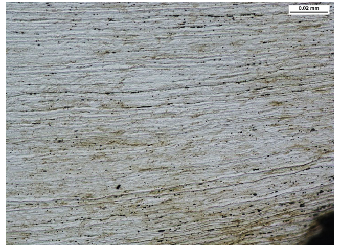
Fig. 12. Microstructure of the baseline sample, LOM, etched in nital
