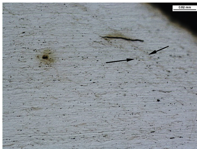
Fig. 14. Microstructure of sample no. 6, LOM, etched in nital
