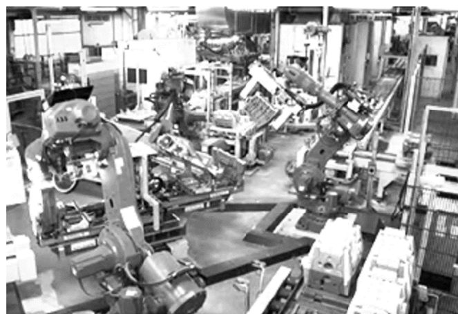
Fig. 1. Automated core and mould assembly [3]
