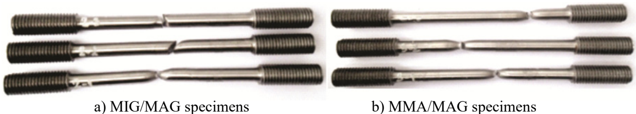
Fig. 12. Specimens with welded joint after testing
