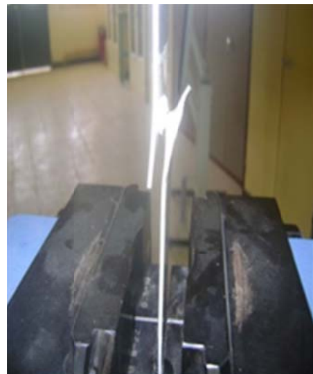
Fig. 11. Shear specimen during the tensile test
