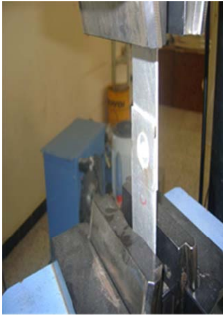
Fig. 5. An example of tensile shear test specimens
