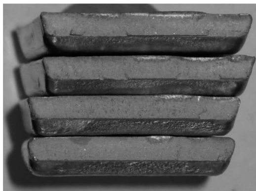
Fig. 7. Examination of fracture on particular parts of sample, cast from melting furnace
