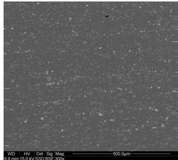
Fig. 6. SEM microstructure of FMP AlSi9Mg alloy at rotational speed of 560 rpm and traverse velocity of 560 mm/min
