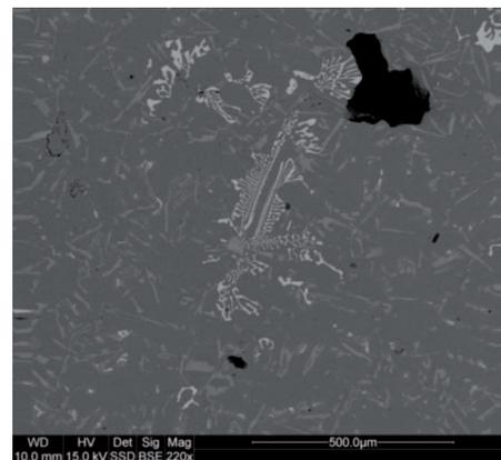
Fig. 3. An example of pores in the microstructure of as cast AlSi9Mg
