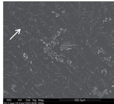
Fig. 2. Microstructure of as-cast AlSi9Mg alloy, Si particle marks by arrow
