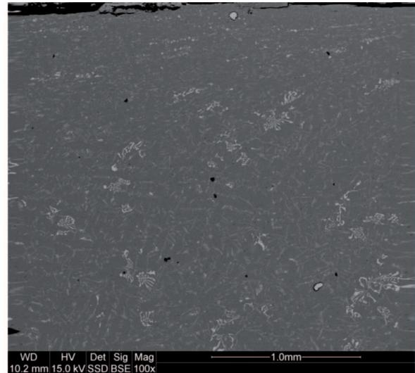
Fig. 5. Typical cross-section of the processed surface layer; SEM
