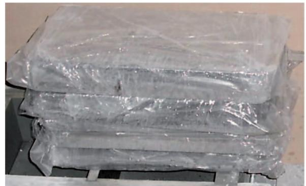
Fig. 2. Plates of formed mould powder for industrial studies
