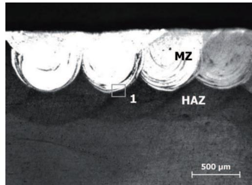
Fig. 1. Microstructure of C45 steel after borochromizing and LHT  $q = 41.40 \text{ kW/cm}^2$ ,  $v = 0.67 \text{ m/min}$ ; Reagent: solution 2% HNO<sub>3</sub>
