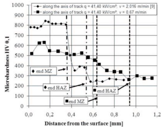
Fig. 5. Microhardness of C45 steel after borochromizing and LHT  $q = 41.40 \text{ kW/cm}^2$ ,  $v = 0.67 \text{ m/min}$ ; and  $q = 41.40 \text{ kW/cm}^2$ ,  $v = 2.016 \text{ m/min}$ ; measure along the axis of track
