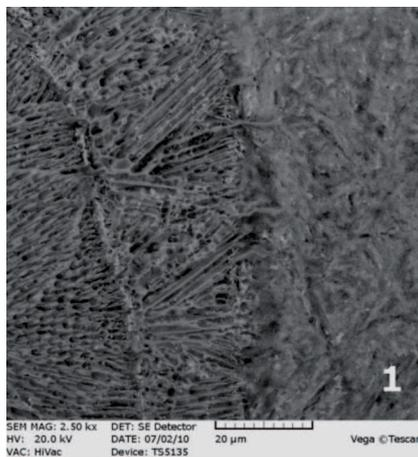
Fig. 4. Microstructure of C45 steel after borochromizing and LHT  $q = 41.40 \text{ kW/cm}^2$ ,  $v = 2.016 \text{ m/min}$ ; boundary MZ and HAZ; Reagent: solution  $\text{CuSO}_4 + \text{HCl} + \text{H}_2\text{O}$  [9]
