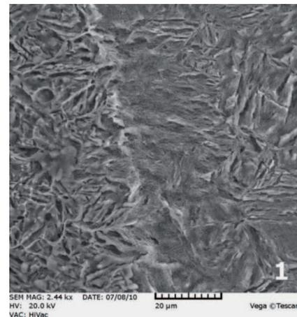
Fig. 2. Microstructure of C45 steel after borochromizing and LHT  $q = 41.40 \text{ kW/cm}^2$ ,  $v = 0.67 \text{ m/min}$ ; boundary MZ and HAZ; Reagent: solution CuSO<sub>4</sub> + HCl + H<sub>2</sub>O
