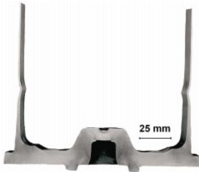
Fig. 6. Image of the macrostructure of Bw11 steel pressed product, without segregation. Longitudinal section after macroetching. Heat no. 517701
