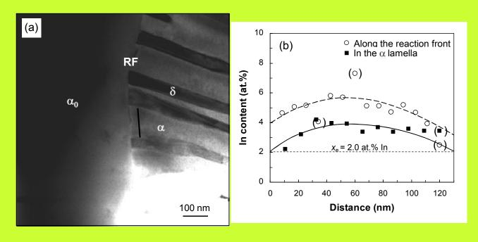
Cu - 7.5 at.% In annealed at 330 °C for 48 h
