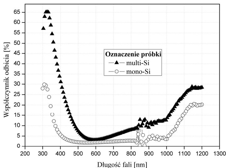
Fig. 4. Reflectance for multi and mono crystalline solar cells
