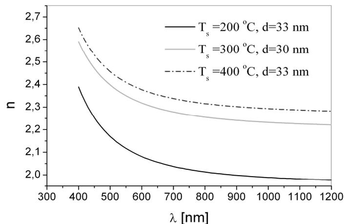
Fig. 3. Refractive index  $n$  as a function of wavelength  $\lambda$ . [1]
