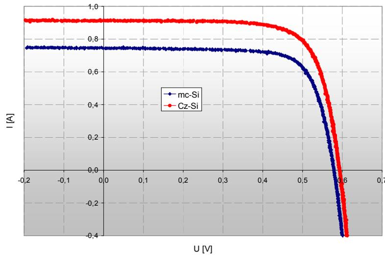
Fig. 6. The measured I-V characteristic for monocrystalline silicon solar cell (Cz-Si) and (mc-Si)
