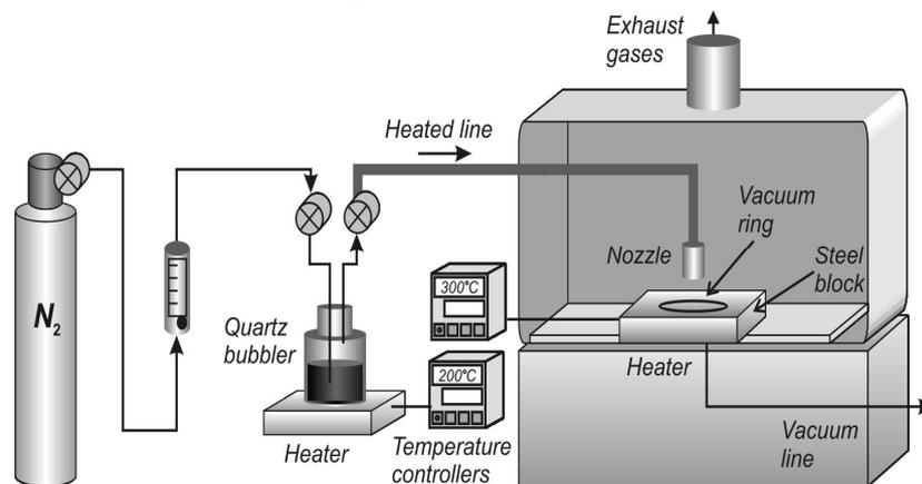
Fig. 1. Scheme of the  $\text{TiO}_2$  antireflection layer deposition system by CVD method.
