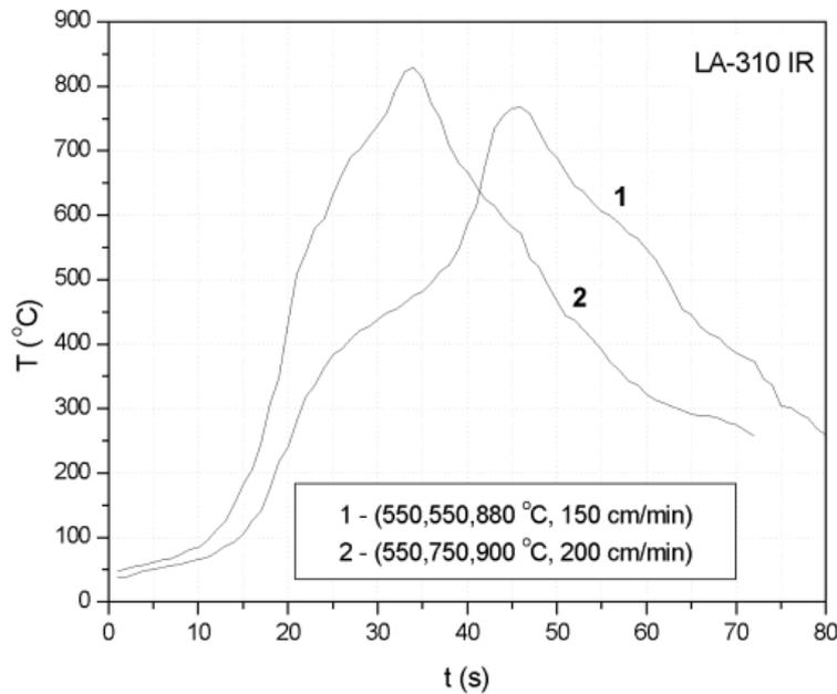
Fig. 5. Temperature profiles vs. elapsed time for solar cell metallisation in the IR furnace.
