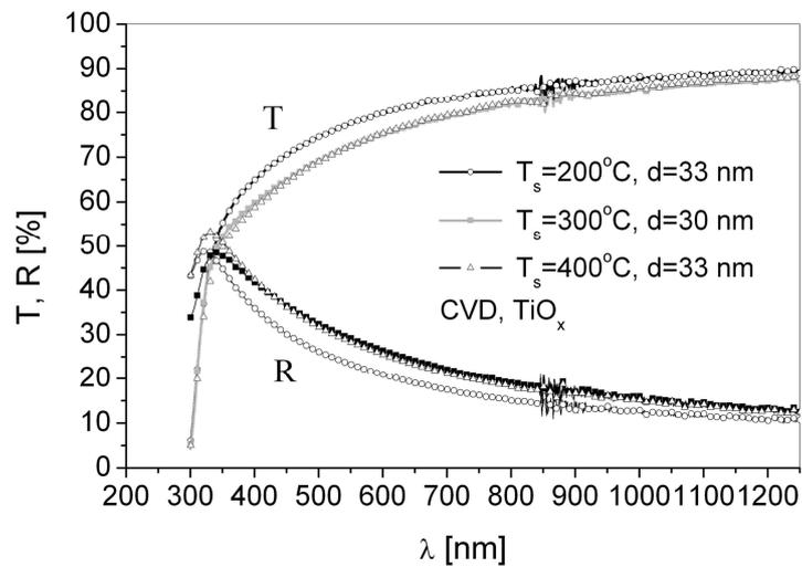
Fig. 2. The influence of the substrate temperature on the optical spectra of  $TiO_2$  layers. [1]
