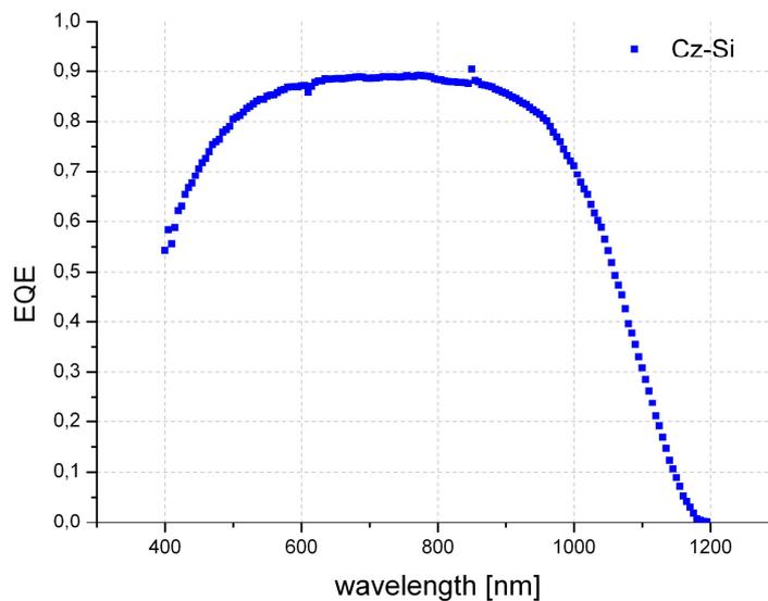
Fig. 7. External quantum efficiency (EQE) for solar cell with SiO<sub>2</sub> passivation layer and TiO<sub>x</sub> ARC
