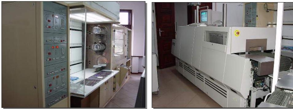
Fig. 2. The industrial furnace for diffusion and heat treatment processes (PIE) and infrared belt furnaces (RTC type LA-310).
