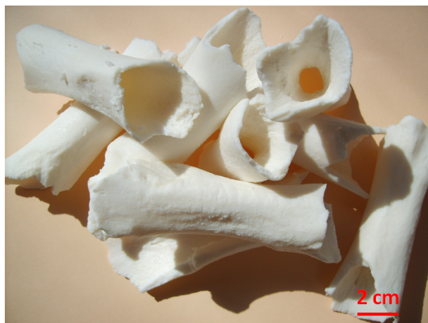
Fig. 1. Cortical part of porcine bones after leaching of organic matter with sodium hydroxide solution.
