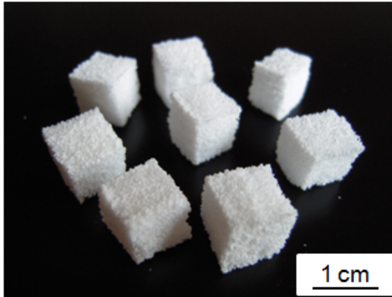
Fig. 4. macroporous ceramics obtained by use of polymer sponge method from porcine origin hydroxyapatite and phosphate glass [Janus, 2010].
