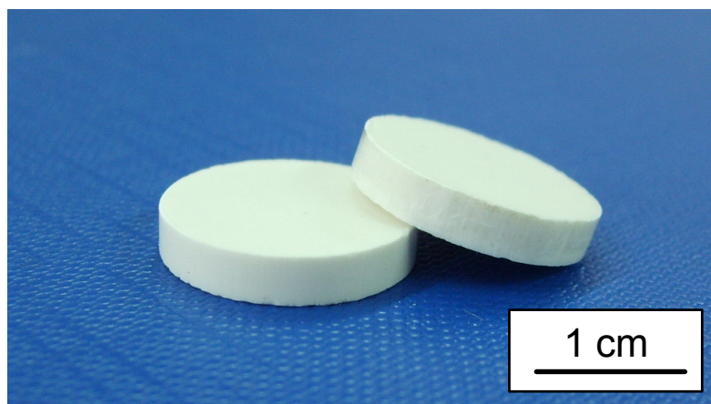
Fig. 2. Dense ceramics prepared from porcine origin hydroxyapatite and sintered at 1200°C [Janus, 2010].
