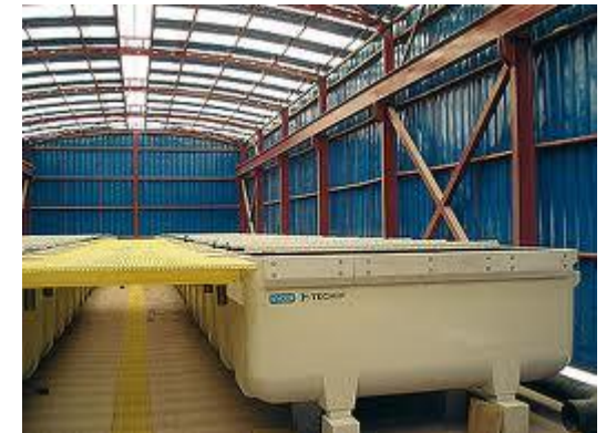
Zinc electrowinning at the Teck Cominco zinc refinery in Trail, BC, Canada
