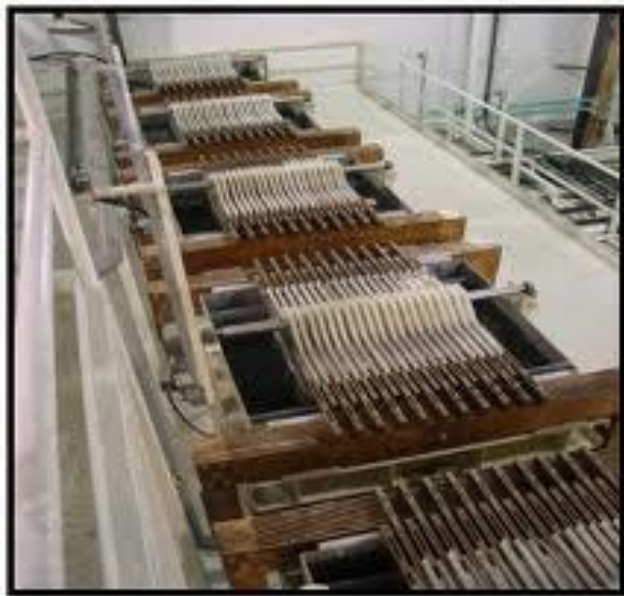
Electrowinning cells for recovery of zinc
